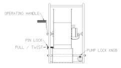
Figure 3: Unlocking Pump Holster Pin
