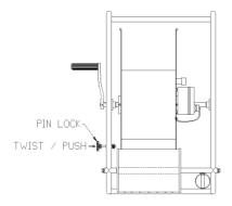
Figure 9: Pin-locking the Reel
