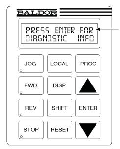
**Keypad Display** - Displays status information during Local or Remote operation. It also displays information during parameter setup and fault or Diagnostic Information.
