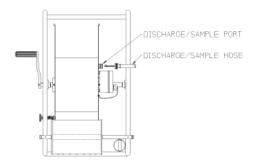
Figure 6: Discharge Ports
