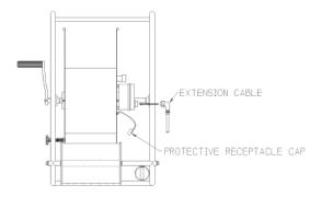
Figure 10: Electrical Connections
