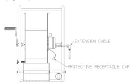
Figure 5: Electrical Connections
