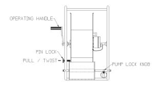
Figure 8: Unlocking the Pin Lock
